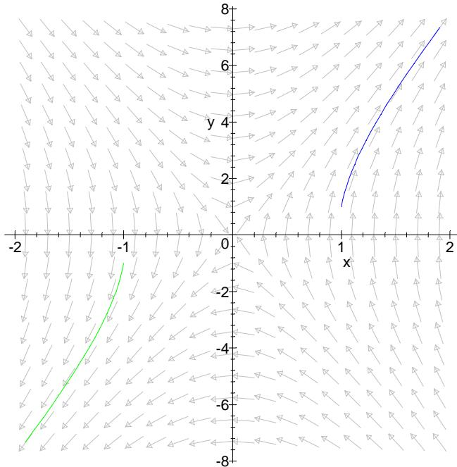
Category 1: Plot is at  $z=0$  for  $t = -1.5$ ,  $m = n$ . The plot is the value of the B field lines at constant  $t$ . These are streamlines not streaklines. The  $x,y$  scales are distorted. This is the evolutionary saddle at early times. Two flow lines are shown for initial conditions of  $[x=1,y=1]$  in blue and  $[x=-1,y=-1]$  in green
