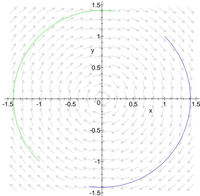
**Category 1:** The plot is a  $z=0$  for  $t=0$  and  $m= - n$ . The plot is of the B field streamlines at a fixed  $t$ . This is the rotational mode at  $t = 0$
