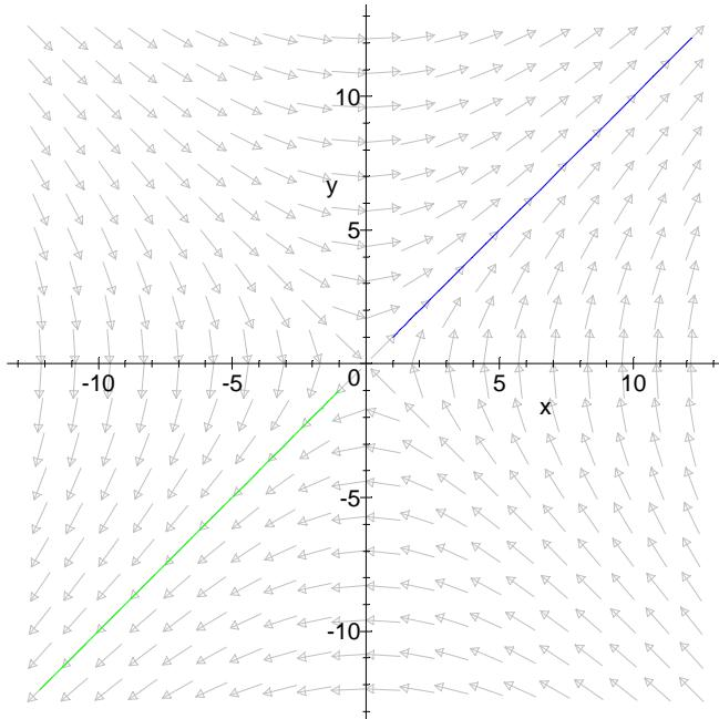
**Category 1:** Plot is at  $z=0$  for  $t=0$ ,  $m=n$ . The plot is the value of the B field lines at constant  $t$ . (stream lines, not streak lines) The  $x,y$  scales are not constrained. This is the evolutionary saddle mode for  $t=0$ . Two flow lines are shown for initial conditions of  $[x=1,y=1]$  in blue and  $[x=-1,y=-1]$  in green
