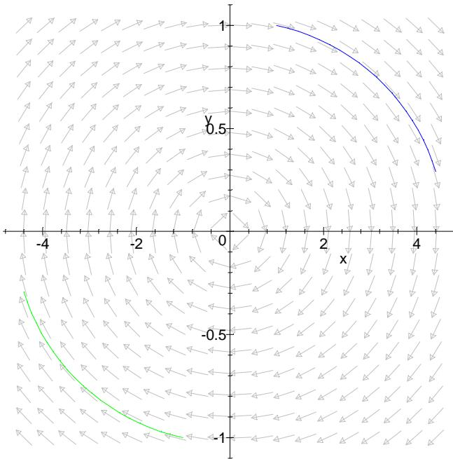
**Category 1:** Plot is at  $z=0$  for  $t=1.5$ ,  $m= - n$ . The plot is the value of the B field lines at constant  $t$ . (stream lines, not streak lines) The x,y scales are not constrained. This is the evolutionary rotational mode for late times  $t > 0$ .
